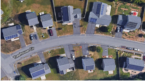
Figure 1: Solar PV arrays are visually identified in publicly-available Google satellite imagery.
